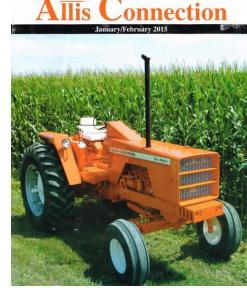
In the fall of 2011, I decided to restore and retire the One-Ninety. I took the Year-Round cab off and installed the original style of fenders. I fixed the few leaks it had and overhauled the engine as it was getting tired. I had the lower block bored and sleeved as it
